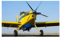
AT-802F Fire Boss - Capable of landing on both water or ground. It can scoop water and then deliver that load to nearby fires. AT-802F Fuel Boss - Can carry up to 4,000 litres at a time of Avgas, Petrol, heating fuel, diesel or Jet A1 to where you need it most, safely and efficiently. Capable of landing on grass or dirt roads and other unimproved airstrips the rugged
